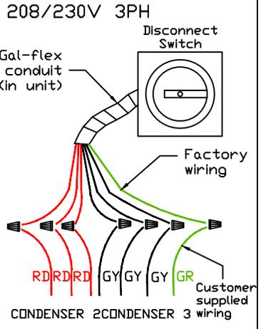
DO NOT CONNECT CONDENSER POWER DROPS TO KITCHEN CONTROL PACKAGE STARTERS OR VFDS
